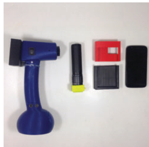
Figure 1: The Mobile Colposcope, disassembled into each of its component parts. From left to right: illumination unit, optical lens assembly, cell phone case, and Motorola Moto G Smartphone.
