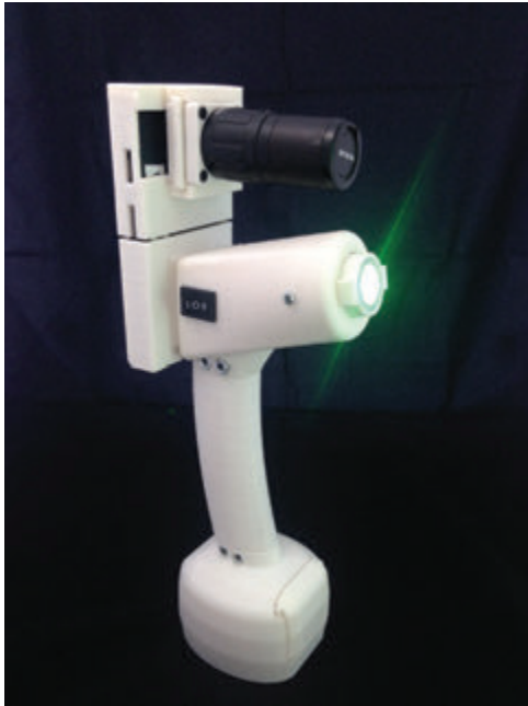
Figure 2: The assembled Mobile Colposcope.
